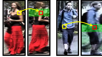
Figure 2. Illustration of adjacency constrained search. Green region represents the adjacency constrained search set of the patch in yellow box. The patch in red box is the target match.
